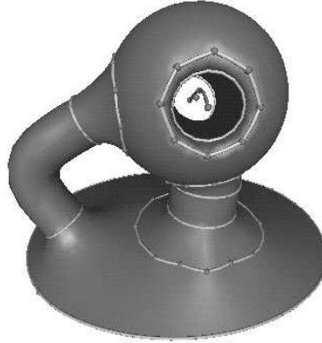
Figure 3.3: A model that mixes variational and explicitly represented shapes. A sphere tool controls a portion of the surface, to which supporting handles have been attached, and through which a hole has been drilled.
