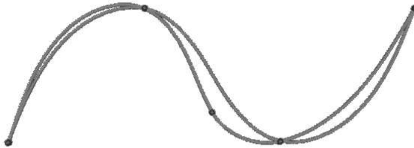
Figure 8.1: Revisiting a curve interpolation problem of Chapter 2: even though the user has grabbed and dragged a point near one of the original interpolation points, the shape remains fair. The success is due to the combination of our geometric thin plate function and adaptive curve sampling.
