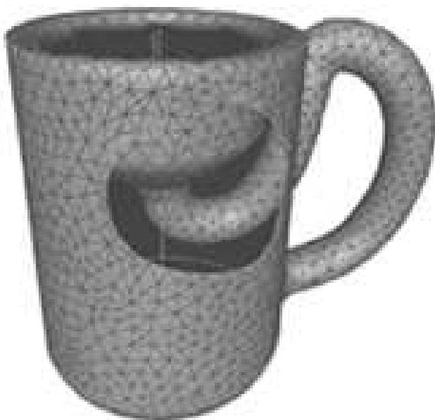
Figure 7.3: A Klein mug , a variation on the famous 1-sided surface. The handle and sidewalls are controlled by cylinder tools. Variational blend surfaces join the cylinders into a globally smooth, non-orientable surface.
